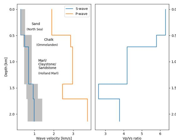
*Figure 1: Left: Inverted S-wave velocity depth profile (blue line) together with publicly available P-wave velocity model. Grey area shows the range of minimum to maximum velocity value at each layer during inversion iterations. Right: Vp/Vs ratio calculated using known P-wave and inverted S-wave velocity.*
