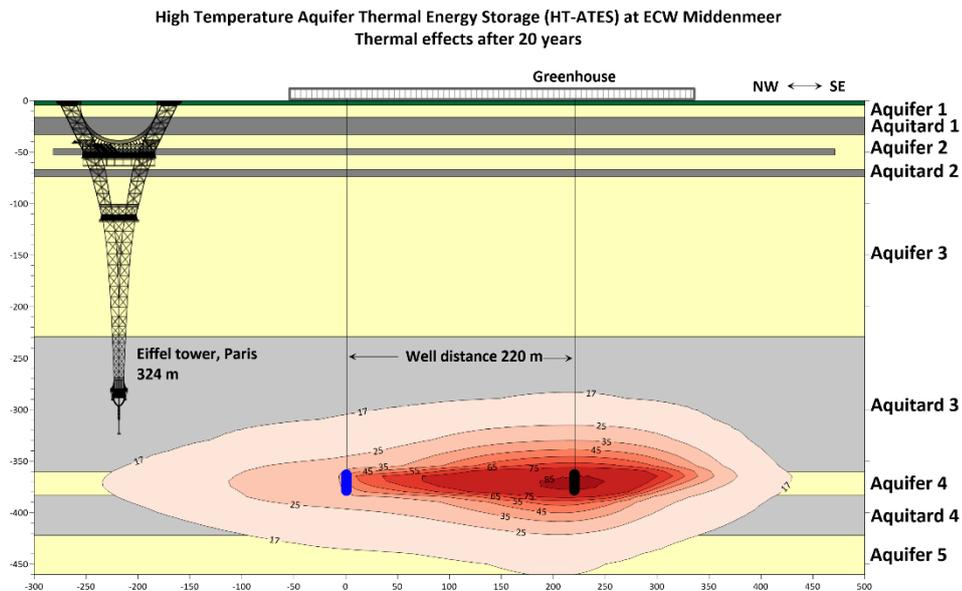
Figure 1: Temperature distribution in the subsurface after 20 years of HT-ATES operation, as estimated by numerical models before operation.
