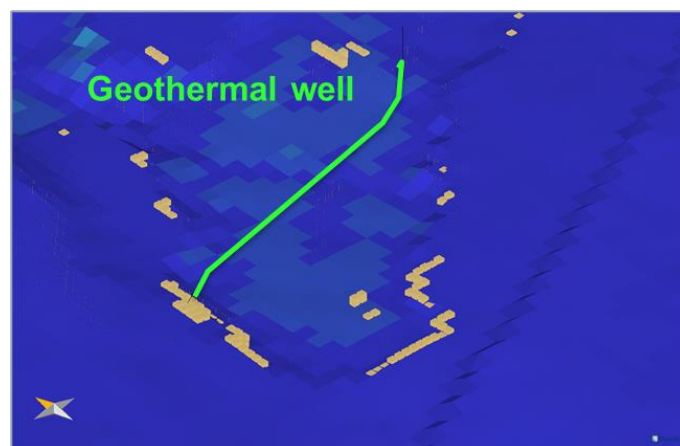
Figure 3: overpressured gas accumulations in the vicinity of a geothermal well (adapted from Omodeo Salè et al. 2020)
