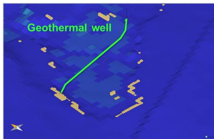
Figure 3: overpressured gas accumulations in the vicinity of a geothermal well
