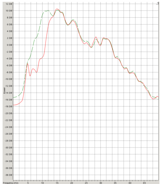
Figure 6: Spectrum after standard subtraction (red) and adaptive subtraction (green, dashed). Note that part of the low frequency content is missing after standard subtraction.
