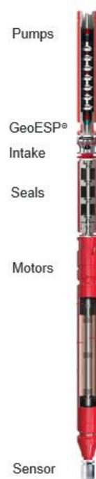
Fig. 1: GeoESP® pump schematic.
