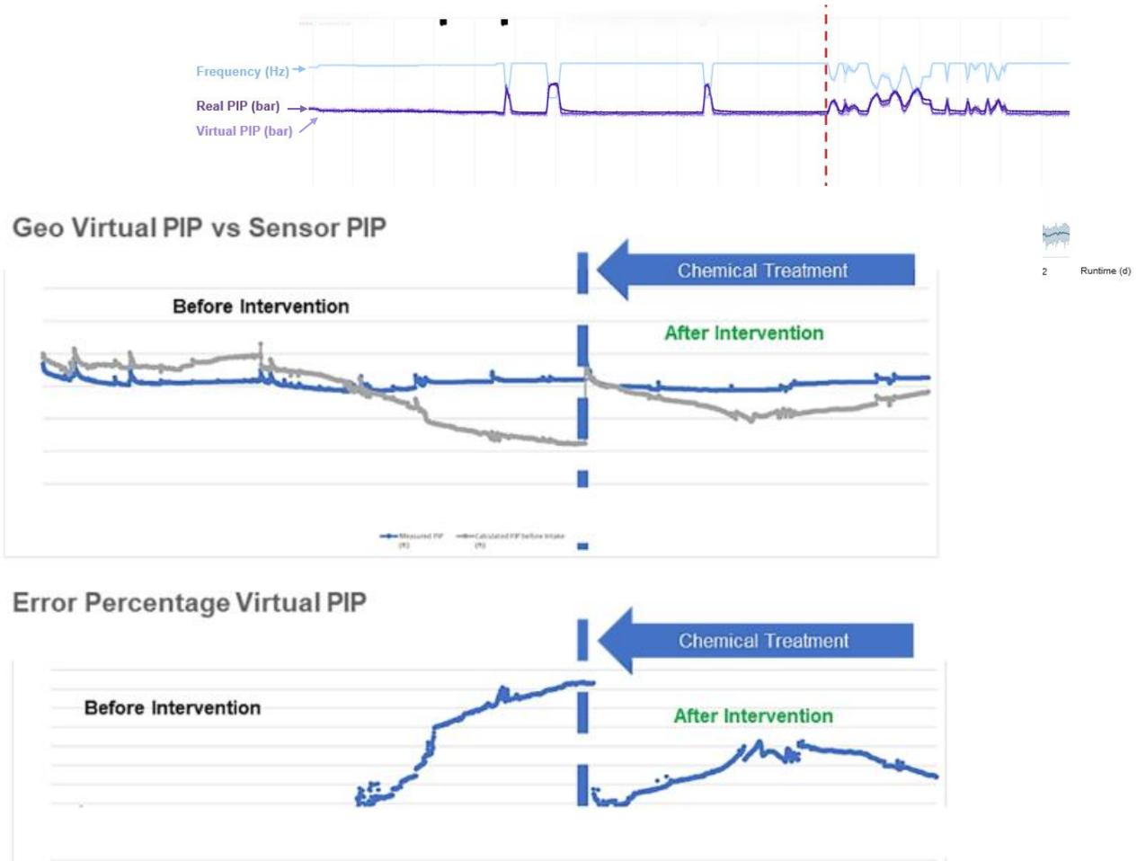
Fig. 6: Proactive chemical treatment based on virtual parameters observations.
