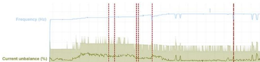
*Fig. 11: A-phase current unbalance tracking during resonance frequencies.*
