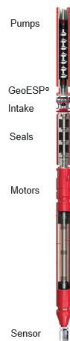
Fig. 1: GeoESP® pump schematic.
