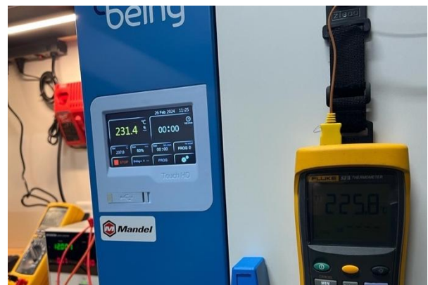
Fig 4: Oven testing above 230°C.
